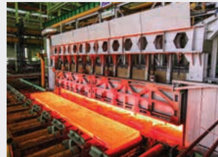
Reheating Furnace of Hot Strip Mill
